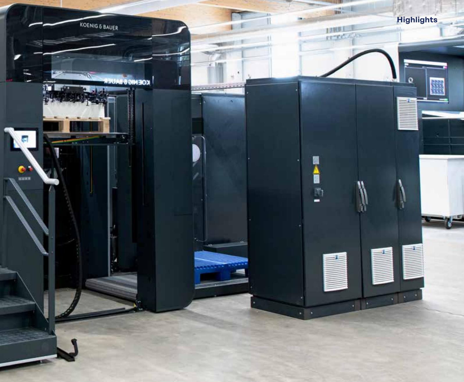
Developed on the basis of the established Rapida-medium<sup>4</sup> format press series, the rotary die<sup>4</sup> cutter CutPRO-X-106 offers you the very latest die<sup>4</sup> cutting technology and a sheer boundless scope of applications. Whether for folding cartons, elegant presentation folders or in mould labels for paint buckets – with the CutPRO-X-106, you can cut, emboss, crease, perforate and then separate the individual blanks to the highest quality standards in a single machine pass.
